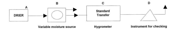
MCM will supply a 2 column heat generated molecular sieve drier (A) that provides particulate fine dry air to the moisture generator (B).
